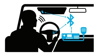
He confirms by voice using the **steering wheel PTT switch and visor mic** connected to his mobile radio via Bluetooth and the dispatcher receives the confirmation through the **MIP 5000 Radio Console.**
